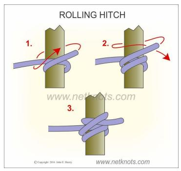
The knot is called the Rolling Hitch. It is a very secure and easy to tie method of fastening a rope to a post and holds firmly in the direction of the standing line. The Rolling Hitch is much more secure than the similar clove hitch when tying a rope to a pole or other object.
